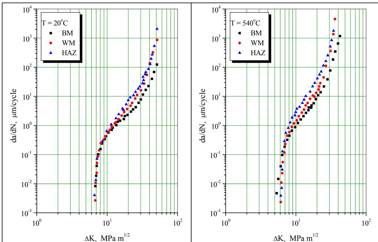
Figure 3. Fatigue crack growth rate per cycle,  $da/dN$ , vs. stress intensity factor range,  $\Delta K$ , specimens pre cracked in BM, WM, and HAY tested at room temperature (left) and at 540 °C (right)
