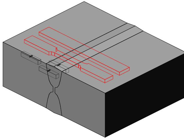
Figure 1. View of testing coupon with double "U" weld and specimens sampling
