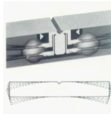
Figure 2. General disposition of RUMUL CRACKTRONIC FRACTOMAT device for fatigue growth rate (left) and view of specimen with cemented foil crack gauge with variable loading bending scheme (right)
