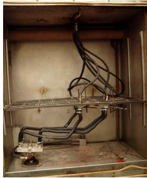
Figure 2. Test chamber and tube samples
