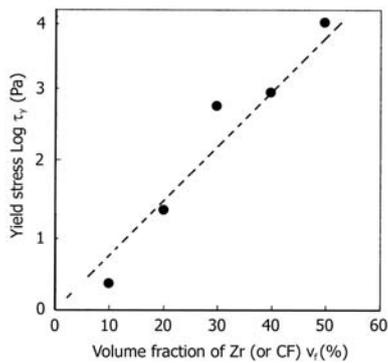
Fig. 1. Relationship between yield stress,  $\tau_y$ , and volume fraction of  $ZrO_2$  powder,  $v_f$ , for Zr/PP melts
