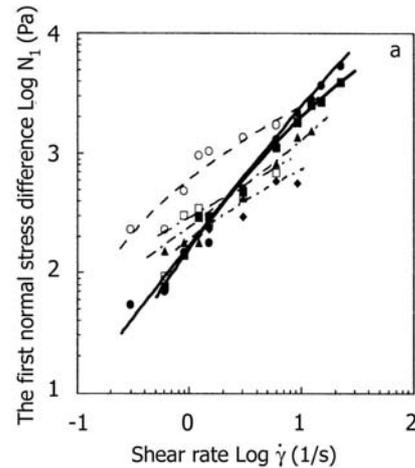
Fig. 2. First normal stress difference,  $N_1$ , as function of shear rate,  $\dot{\gamma}$ , for PP (■), Zr10/PP (●), Zr20/PP (▲), Zr30/PP (◆), Zr40/PP (□), Zr50/PP (○) melt.
