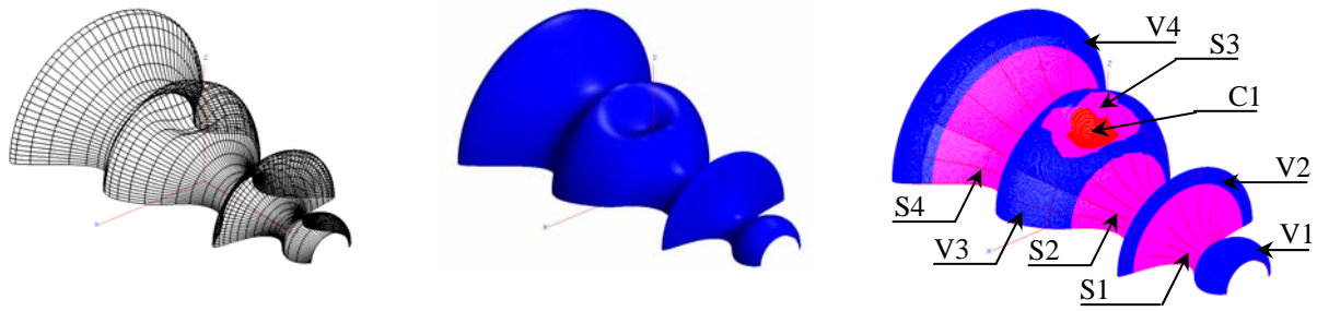
a. Wireframe model of the surface. b. Shaded model of the surface. c. Sub regions of the surface.
