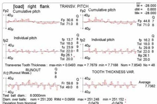
Figure 5. Run out and pitch evaluation chart
