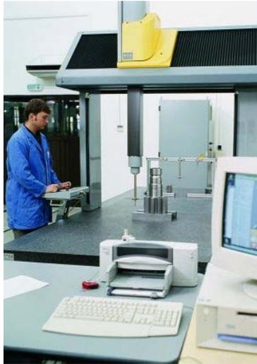
Figure 3. Measurement of worm wheels for cylindrical worms on Brown&Sharpe ghibli-trax
