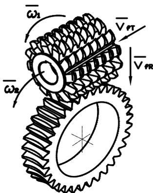
Figure 1 Position and relative motions of worm gear VGM
