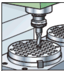
Figure 1. Process of hole making
