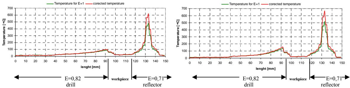
Figure 4. Temperature distribution along axis of driller for working data ( $E=1$ ) and corrected data for first and second hole
