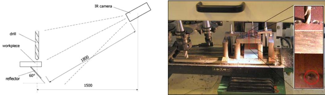
Figure 1. The temperature measuring stand
