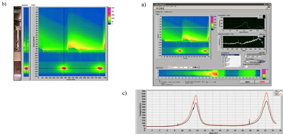
Figure 3. a) main window of application for termovision images sequence analysis; b) view in visible range and IR range of driller top and linear temperature distribution of driller axis with respect to time; c) reflector temperature with respect to time  $T_r=f(t)$  during the drilling of two holes: T1 – temperature at  $E=1$ , T2 -  $E=0,71$
