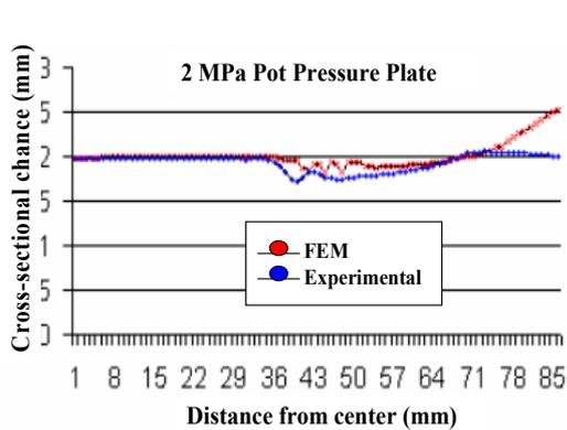
Figure 4. Thickness changes in ANSYS LS-DYNA and specimen for 2 MPa
