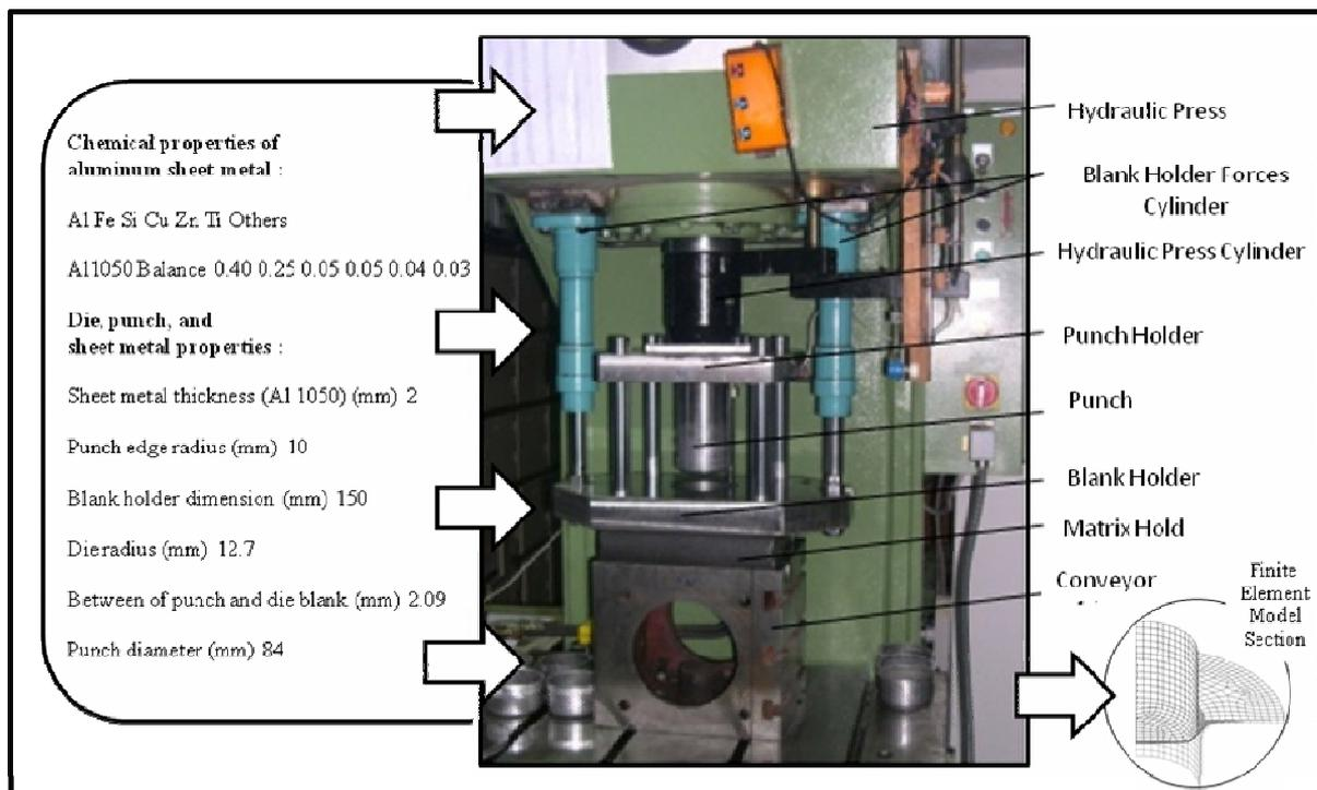
Figure 1. Deep drawing operation machine (hydraulic press and its elements)
