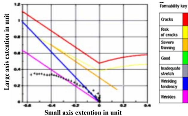
Figure 5. Limit diagram for 2 Mpa Blank holder force
