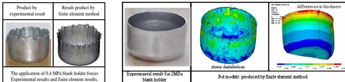
Figure 3. Sheet metal drawing experimental and FEM results for Al 1050 alloy
