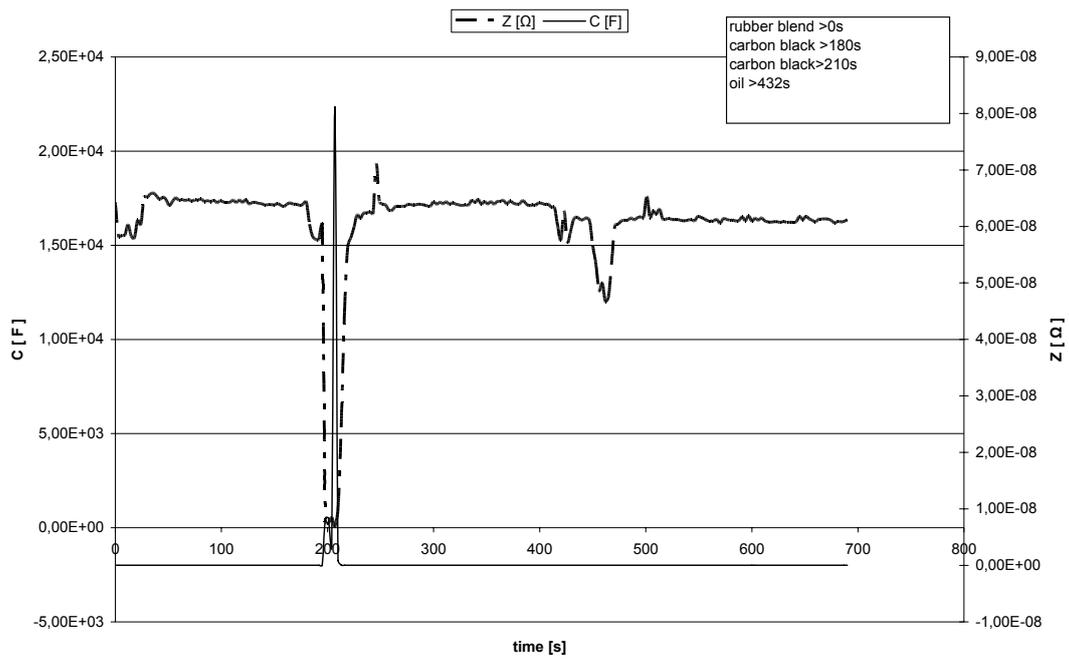
Figure 1. The dependence of the impedance and capacity versus time for the sample 1
