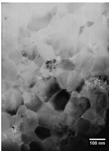
Figure 3. Transmission electron micrograph of Nd_{14}Fe_{79}B_7 alloy after thermomagnetic measurement with grain size distribution
