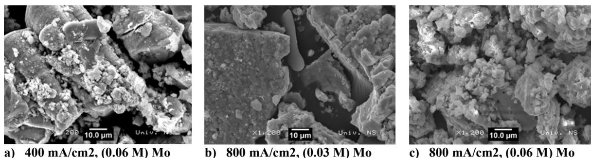
Figure 1. SEM micrographs of Co-Ni-Mo-O alloy powders, electrodeposited from the solution containing  $\text{Ni}^{2+}/\text{Co}^{2+}$  (1:1) concentration ratio [0.1M Ni, 0.1 M Co]
