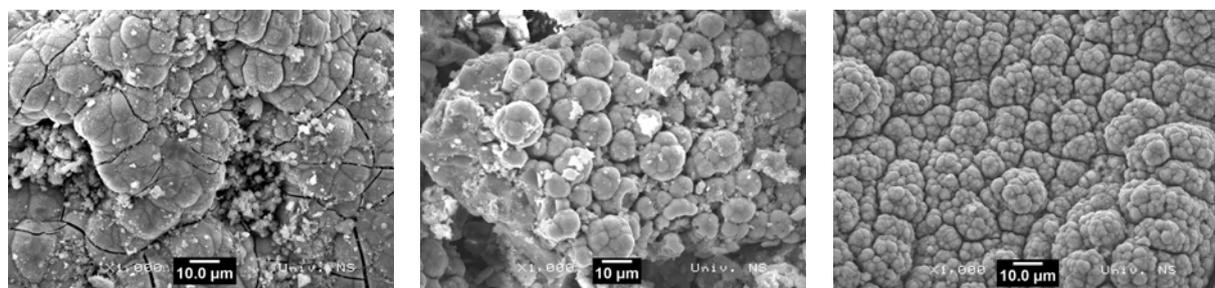
Figure 2. SEM micrographs of Co-Ni-Mo-O alloy powders, electrodeposited at the current density of  $400 \text{ mA/cm}^2$  from the solution containing  $\text{Ni}^{2+}/\text{Co}^{2+}$  (4:1) concentration ratio [0.16M Ni, 0.04 M Co]
