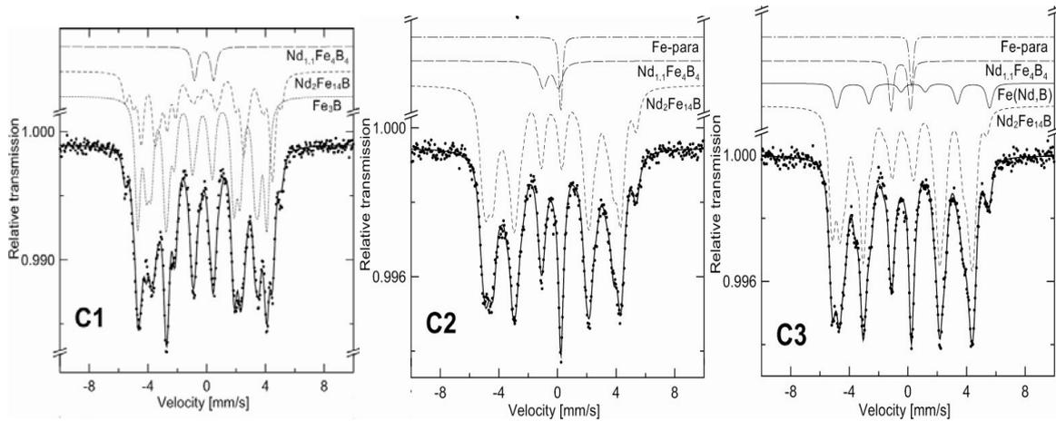
Figure 2. Mossbauer phase analysis of the Nd-low-C<sub>1</sub>, stoich-C<sub>2</sub>, and Nd-rich –C<sub>3</sub> alloys
