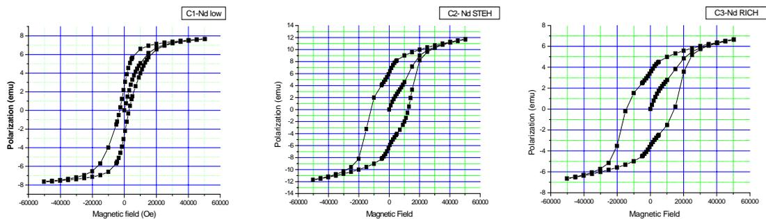
Figure 3. Hysteresis loops for three investigated Nd-Fe-B alloys
