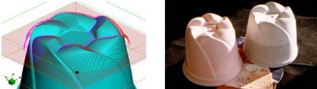
Figure 1. Final product manufactured by using the milling strategy designed in SurfCAM system – raster toolpath copying the shape
