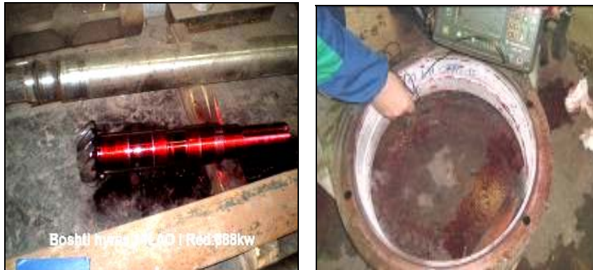
Figure 4. Details controlled by liquid penetrant and ultrasound
