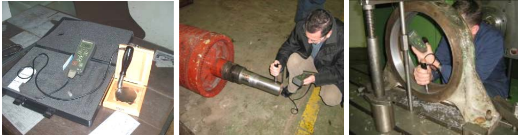
Figure 2. Unit MIC Krautkramer and the way of measurement of the hardness of different details
