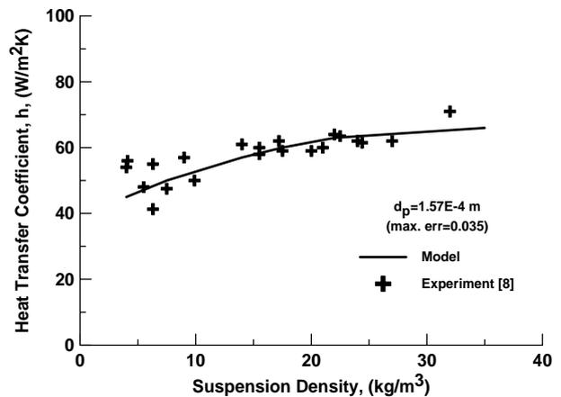
Figure 2. Effects of suspension density on bed-to-wall heat transfer.
