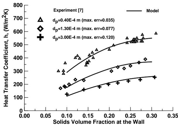
Figure 1. Effects of solids volume fraction on bed-to-wall heat transfer.
