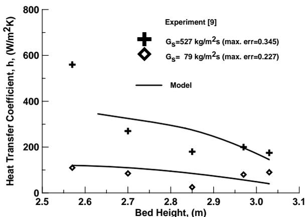
Figure 3. Effects of solid circulation rate on bed-to-wall heat transfer.
