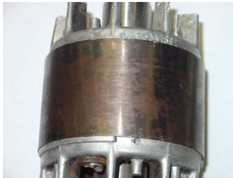
Figure 4. Induction motor with a broken rotor bar
