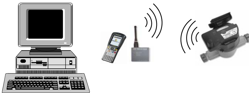
Figure 4. Schematic show of Radio meter reading
