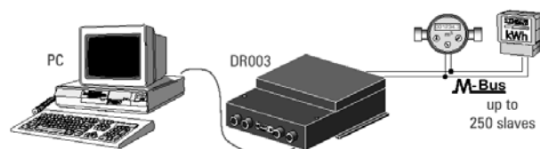
Figure 1. Schematic show of water meter connection to M – bus Digitam master in network up to 250 slaves
