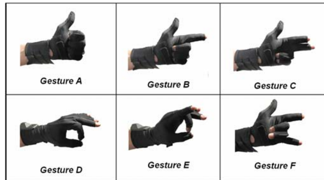
Figure 1. An extended set of gestures which employ thumb for 5DT Ultra 5 data glove
