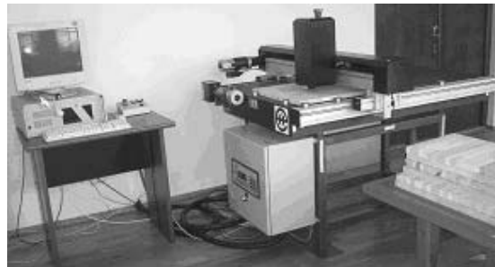
Figure 5. The OptoDESQ table used to measure the depth in the points indicated for each panel type
