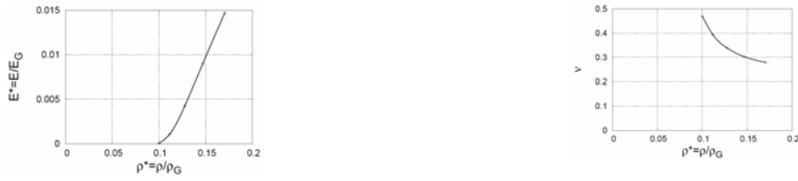
Figure 6. Dependence of relative elastic modulus a) and Poisson ratio b) on relative density of trabecular tissue
