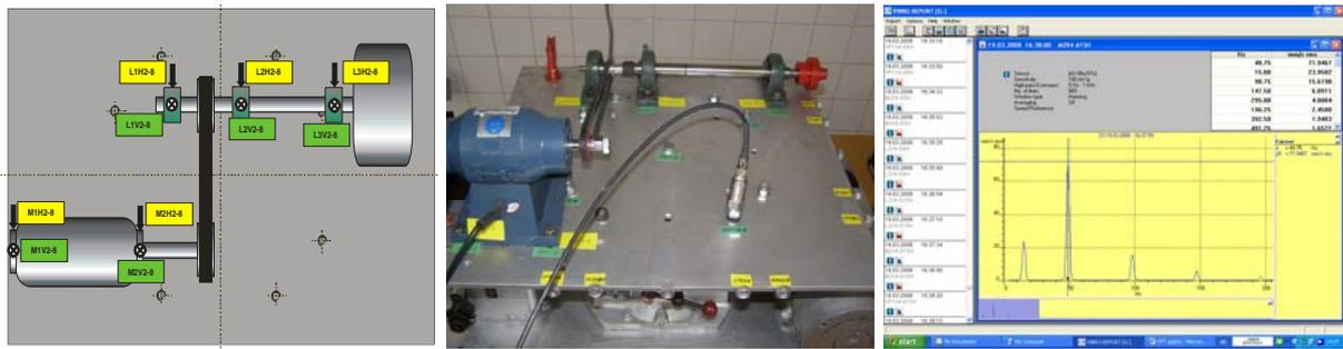
Figure 2. a) Scheme; b) Photography EXM-SVI8; c) FFT spectrum at the specific location
