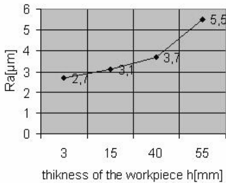
Figure 4. The diagram of roughness variation depending on the thickness of the work piece
