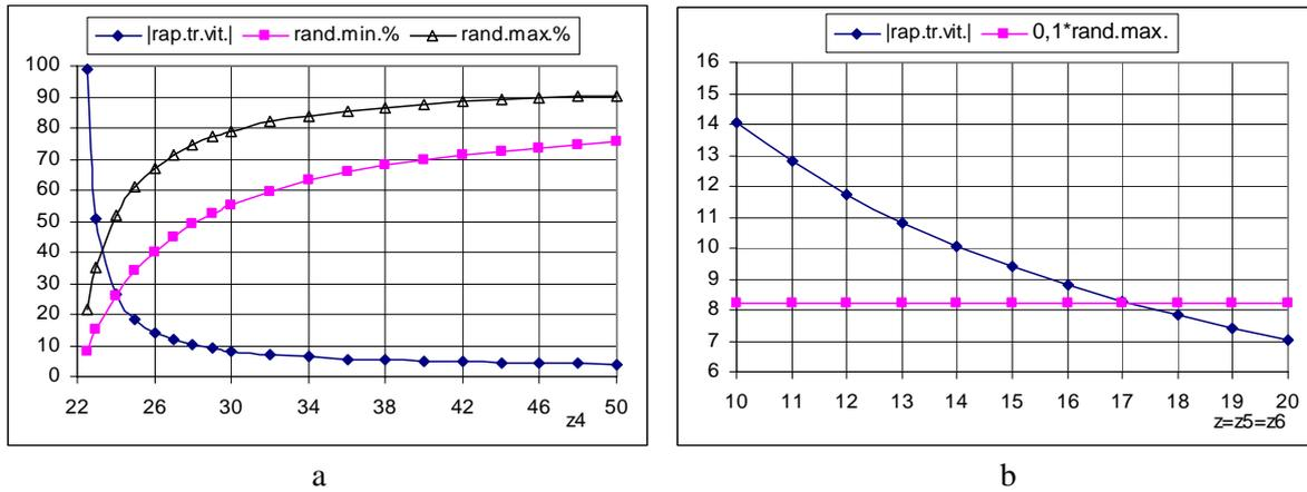
Figure 2. The diagrams for the variation of the transmission ratio module  $|i_{a,H}|$  and of the efficiency  $\eta_{a,H}$ : a) in terms of the teeth number  $z_4$  (the diagram *rand.min.* was obtained in the premise that  $\eta_{01} = 0,94^2 \cong 0,883$  and  $\eta_{02} = \eta_{03} = 0,94$ , and the diagram *rand.max.* was obtained in the premise that  $\eta_{01} = 0,98^2 \cong 0,96$  and  $\eta_{02} = \eta_{03} = 0,98$ ); b) in terms of the teeth number  $z = z_5 = z_6$ .
