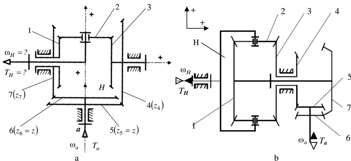
Figure 3. a) Scheme of the initial Vaucanson's planetary reducer; b) Vaucanson variant, optimized on the basis of the paper conclusions, which can be used either as speed amplifier or as speed reducer.
