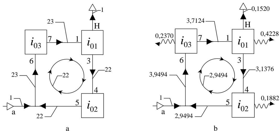
Figure 1. The circulation of the power branches in the Vaucanson planetary reducer: a) the scheme of the power circulation, while neglecting friction; b) the scheme of the power circulation, while considering friction.
