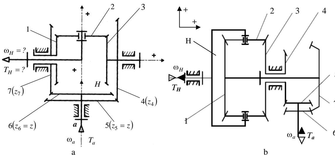
Figure 3. a) Scheme of the initial Vaucanson's planetary reducer; b) Vaucanson variant, optimized on the basis of the paper conclusions, which can be used either as speed amplifier or as speed reducer.
