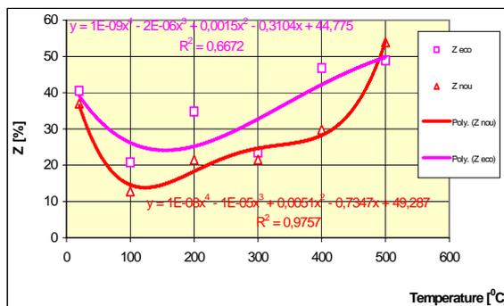
Figure 7. Variation of the Z value, with the temperature, for OLT 45K, in two alternatives of utilization
