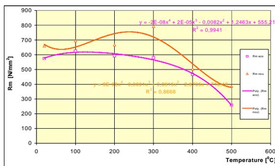
Figure 5. Variation  $R_m$  with the temperature, for OLT 45K steel, in two alternatives of utilization
