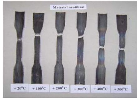
Figure 4. Specimen for testing, drawn from the unused material
