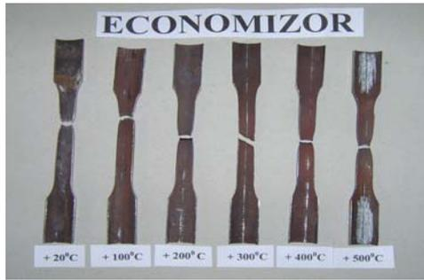
Figure 3. Specimen for testing, drawn from the economizer's material
