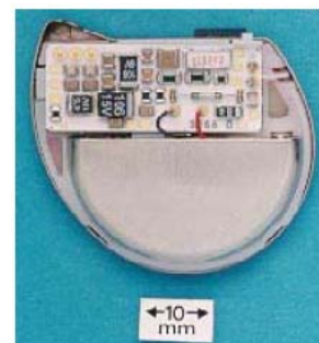
Figure 4. Medical device containing electronic components [20]
