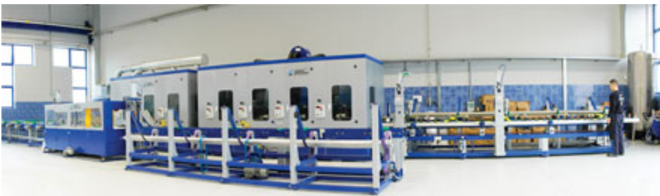
Figure 3. The entire machine for grinding and polishing of circular stainless steel tubes
