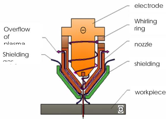
Figure 1. High definition plasma cutting
