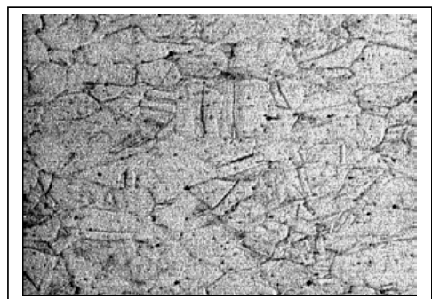
Figure 2. Steel Nitronic 60 (x145), Austenite without \delta ferrite
