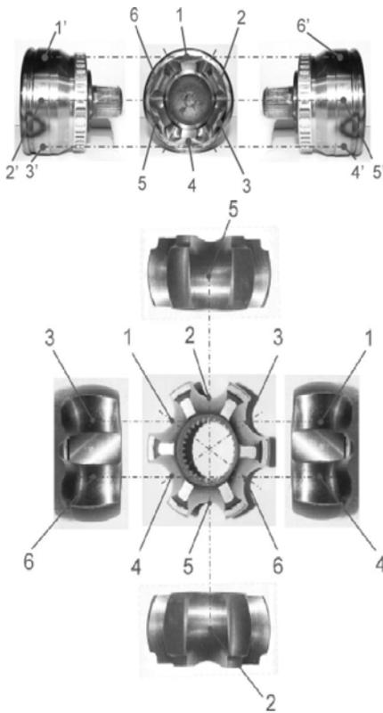
Figure 3. The twelve points where the hardness measurements have been performed on (a) the outer and (b) inner races.
