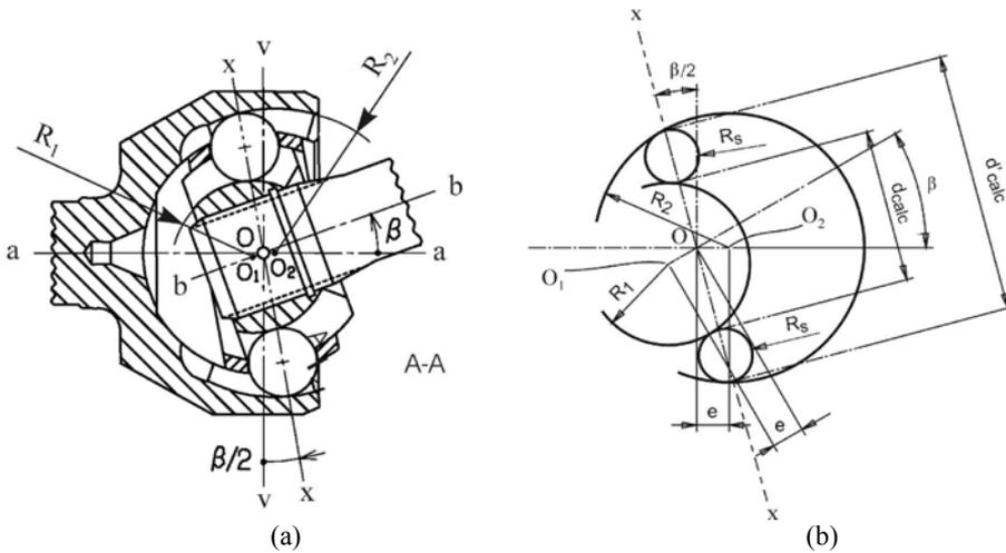
Figure 1. (a) Radii  $R_1$  and  $R_2$  of the grooves defined in the inner and outer races of an Rzeppa constant velocity joint; (b) distances  $d_{calc}$  and  $d'_{calc}$  evaluated by the CAD model.
