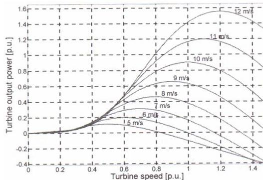
Figure 2. Wind turbine power characteristic.
