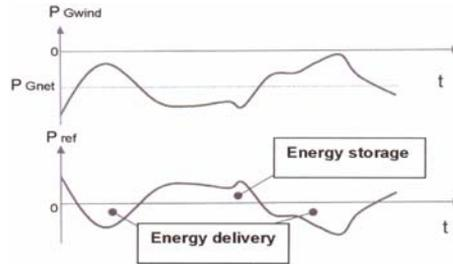
Figure 3. Waveforms to control the system flywheel -wind generator.
