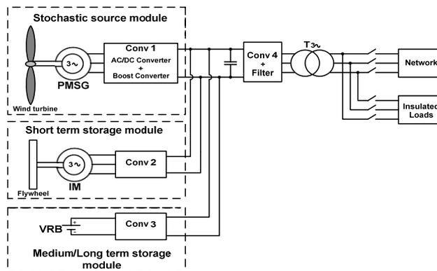
Figure 1. Block diagram of the SSMS for wind systems.
