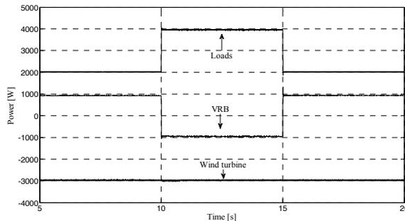
Figure 4. Power balance of the system provided by the VRB.
