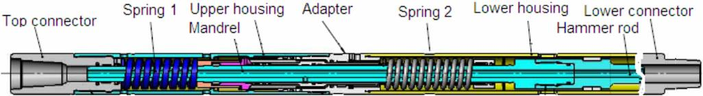
Figure 1. Pictorial section (partial) of the DTH® showing the main components, adapted from [3]
