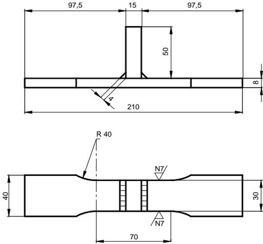
Figure 1. Test specimen
