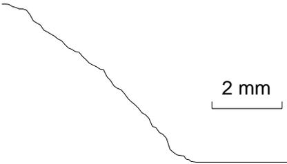
Figure.2. Fillet weld profile
