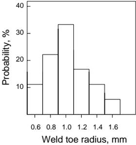
Figure.3. Distribution of fillet weld toe radii
