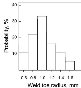
Figure.3. Distribution of fillet weld toe radii
