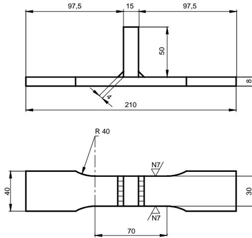
Figure 1. Test specimen
