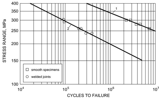
Figure 5. Experimental results and S-N curves for: 1-smooth specimens; 2- welded joints
