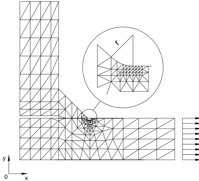
Figure 4. Finite element mesh for one half of the non-load carrying, fillet-welded transverse stiffener
