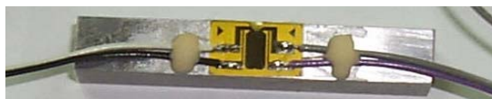
Figure 1. Charpy specimen instrumented by foil RUMUL RMF A-5 for continuous monitoring of crack length
