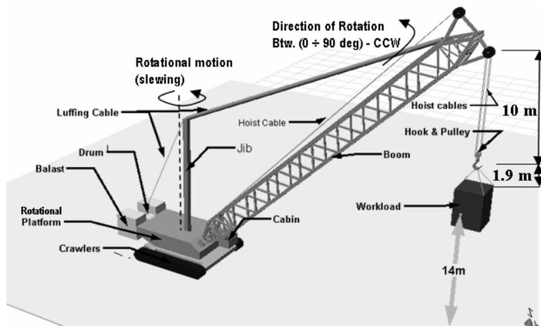
Figure 1. Virtual model of the crawler crane with key elements
