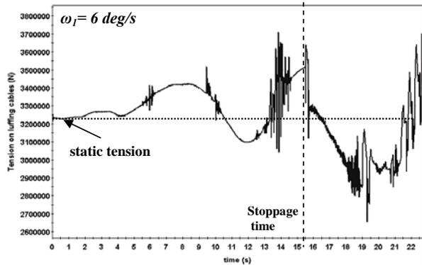
Figure 9. Tension on the cables at  $\omega_1 = 6 \text{ deg/s}$
