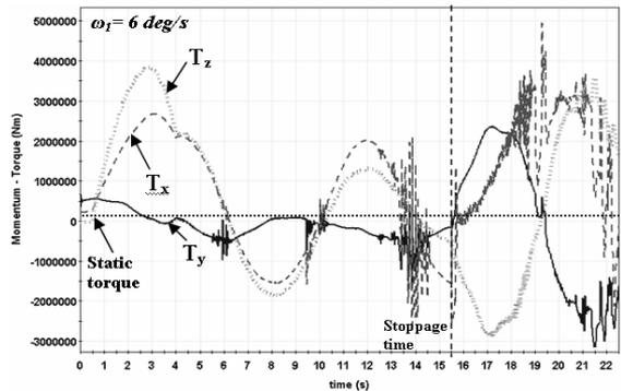
Figure 6. Torque – with rotation at  $\omega_1 = 6$  deg/s
