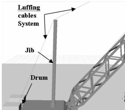
Figure 8. Luffing Cables system
