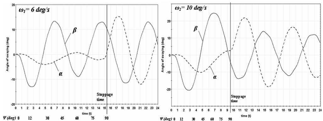
Figure 4. Angles  $\alpha$  and  $\beta$  of workload's swaying around vertical axes
