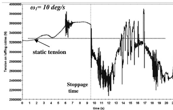
Figure 10. Tension on the cables at  $\omega_1 = 10 \text{ deg/s}$
