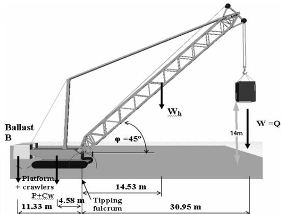
Figure 3. Crane dimensional parameters
