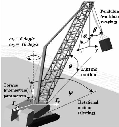
Figure 2. Crane simulation parameters
