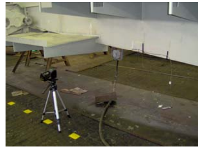
Figure 8. Measurement points at main girders; a) positions, b) realistic view
