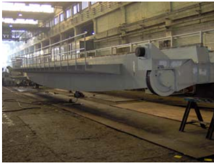
Figure 1. Double girder bridge crane; a) realistic view, b) cross section
