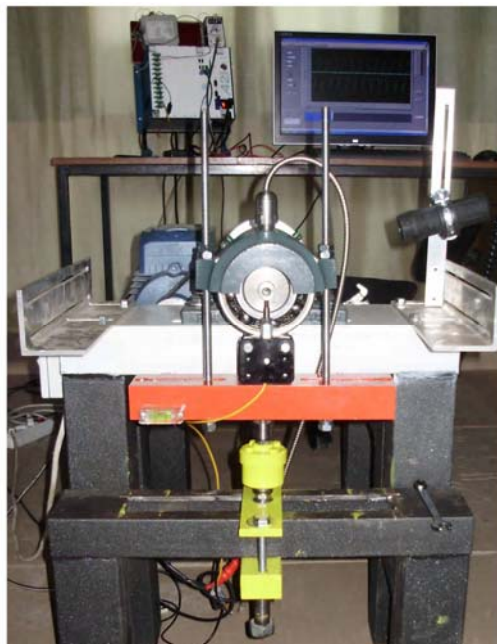
Figure 2. Device for rolling bearings dynamic research
