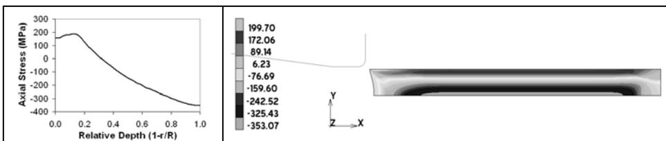
Figure 2. Axial stresses along the section.
