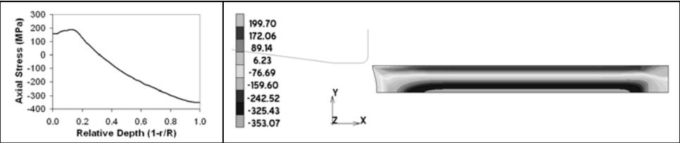
Figure 2. Axial stresses along the section.
