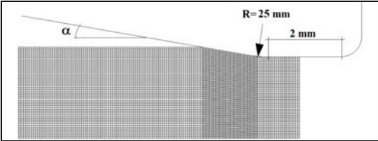
Figure 1. Die geometry and design factors selected.
