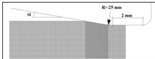
Figure 1. Die geometry and design factors selected.
