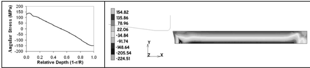
Figure 5. Angular stress along the section.
