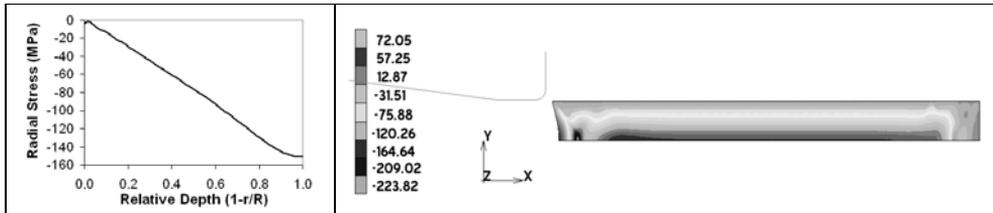
Figure 4. Radial stresses along the section.
