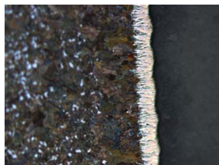
Figure 4. Duplex layers on the steel 42CrMo4
