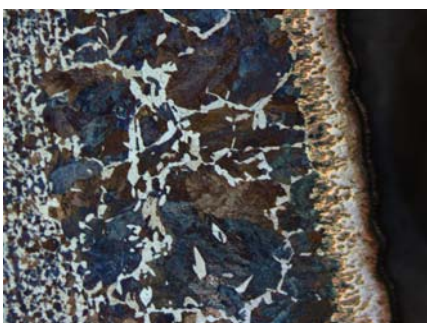
Figure 3. Duplex layers on the steel C45E
