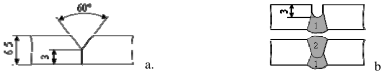
Figure 1. a. Sketch of the welding groove, b. Sketch of the weld and welding layers
