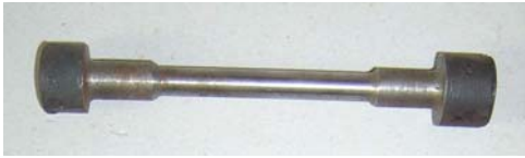
Figure 1. The shape and size of test-bars used in testing
