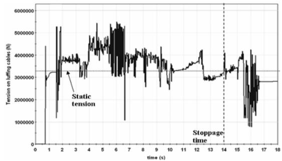
Figure 9. Tension in luffing cables –speed  $v = 0.5 \text{ m/s}$
