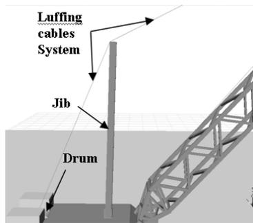
Figure 8. System of luffing Cables
