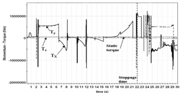
Figure 11. Torque – with speed of  $v = 0.3 \text{ m/s}$
