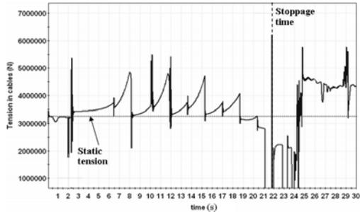
Figure 13. Tension in luffing cables – speed  $v = 0.3$  m/s
