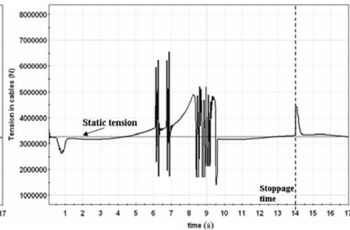
Figure 5. Tension in cables –speed  $v_2 = 1$  m/s
