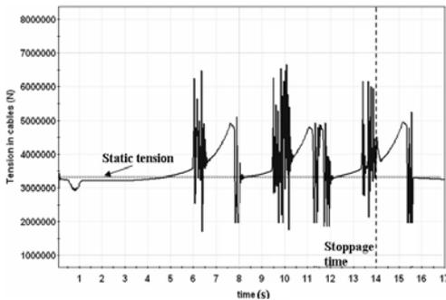
Figure 4. Tension in cables –speed  $v_1 = 0.5$  m/s
