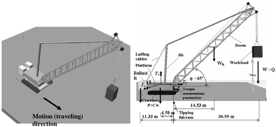
Figure 1. Virtual model of the crawler crane with key elements
