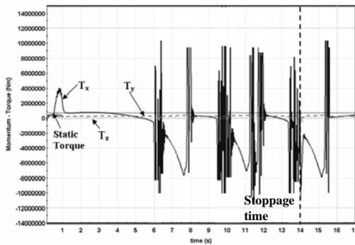
Figure 2. Torque – with speed of  $v_1 = 0.5$  m/s
