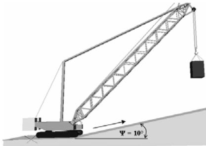
Figure 6. Traveling upwards, angle  $\psi = 10^\circ$
