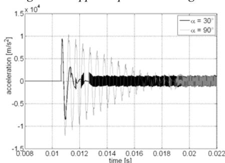
Figure 7. Poppet acceleration diagram
