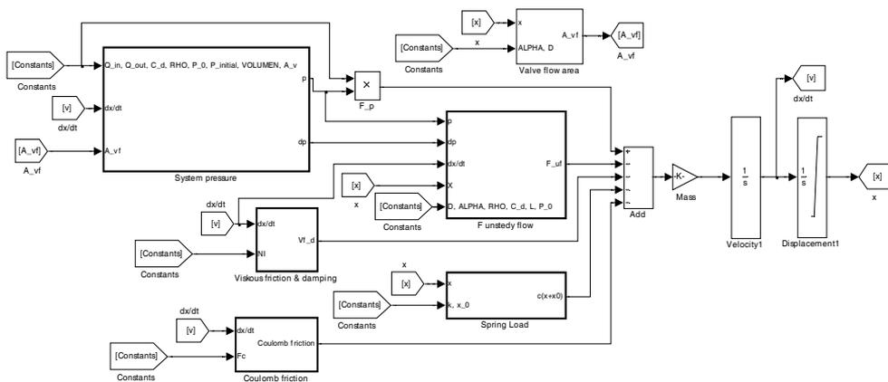
Figure 3. Simulation model of the direct spring operated pressure relief valve
