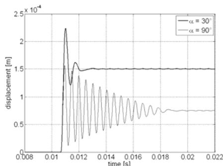
Figure 5. Poppet displacement diagram
