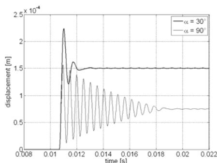
Figure 5. Poppet displacement diagram
