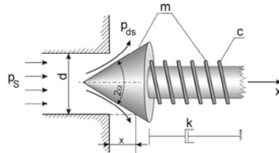
Figure 2. Pressure relief valve model
