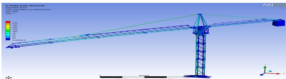
Figure 3. Stress distribution on the tower crane.
