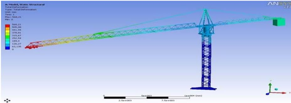
Figure 4. Deformation on the tower crane
