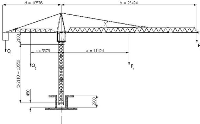
Figure 1. The dimensions of the crane and the loading case
