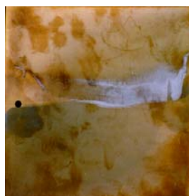
Figure 2. macrophotos of cathode back sides from the Hull cells from organic complex
