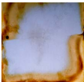
Figure 1. macrophotos of cathode back sides from the Hull cells from cyanide solution
