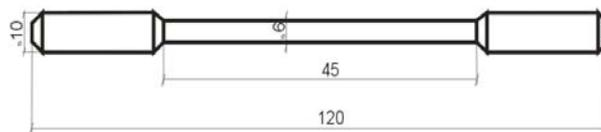
Figure 1. Size of sample for tensile test.
