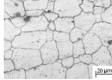
Figure 15. Structure of the sample E- after hot pressing
