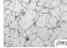
Figure 16. Structure of the sample E- after tensile test
