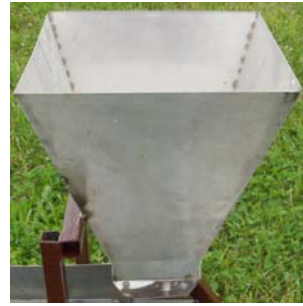
Figure 2. The bunker for granular material
