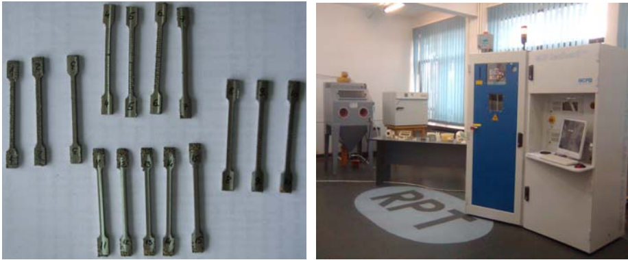
Figure 2. Samples manufactured at the Technical University of Cluj-Napoca on the SLM equipment
