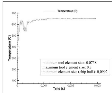
Figure 4. Cutting temperature by standard 3D finite element modeling
