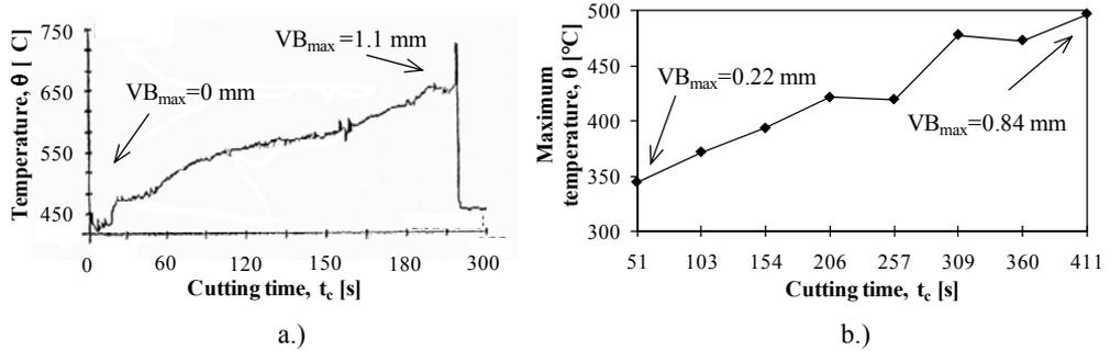
Figure 2. Measured temperatures by optic fibre method (a) and infrared camera (b)
