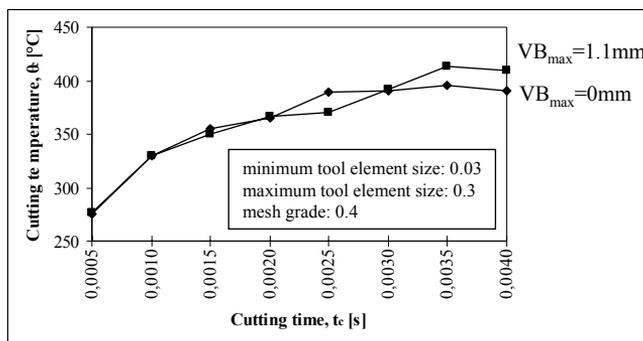
Figure 3. FEM results of cutting temperatures besides different tool-wears
