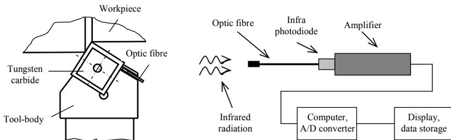
Figure 1. Layout and structure of the temperature measurement (optic fibre method) [6]
