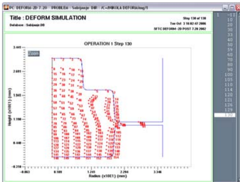
Figure 3. Point arrangement in 13 th phase obtained by DEFORM simulation for convex die
