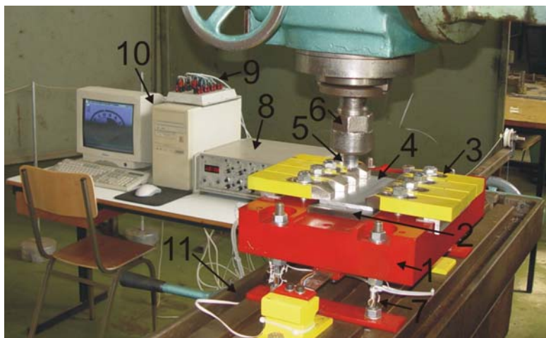
Figure 2. Research site: 1- The base plate, 2 - Support plate, 3 - Work piece clamp, 4 - Work piece of Al alloys, 5 - Tool for FSW, 6 - Clamp part of the milling machines, 7 - Special carrier with glued measuring tapes, 8 - Measuring bridge, 9 - BAS, 10 - PC with A/D card and software GLOBAL LAB, 11 - Work table of milling machine
